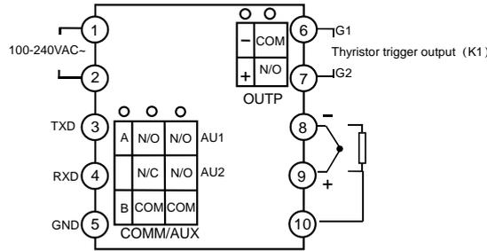
Note 1: D2 dimension instruments don't support 0~5V or 1~5V linear voltage input. However, 0~5V or 1~5V signal can be converted to 0~500mV or 100~500mV by connecting external precise resistors, 4~20mA can be converted to 100~500mV by connecting a 25ohm resistor, then be inputted from terminals 9 and 8.
