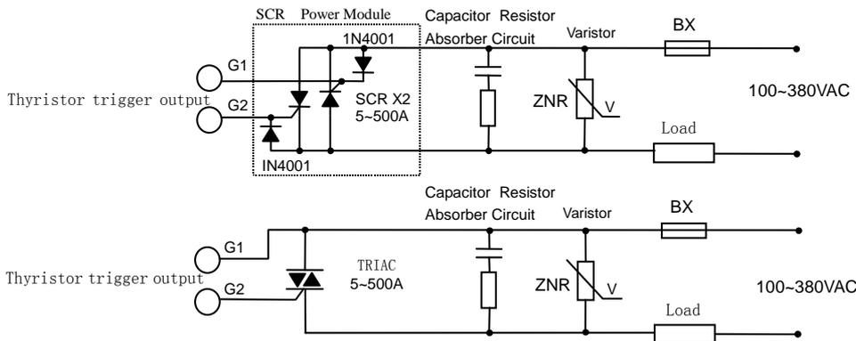
Note 1: According to the voltage and current of load, choose suitable varistor to prevent the thyristor. Capacitor resistor absorber is needed for inductance load or phase-shift trigger output.
