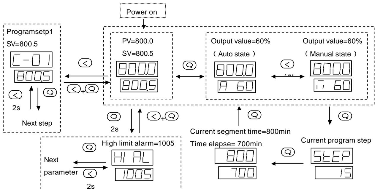
**Note:** Not all types of instruments have the display status shown above. AI-708 has the status of and ; AI-808 has the status of , and ; while AI-808P has all of the display status list above.
