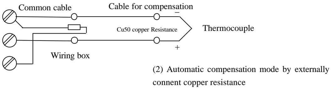
**Note: wiring box should be well way from the heat generating project,
