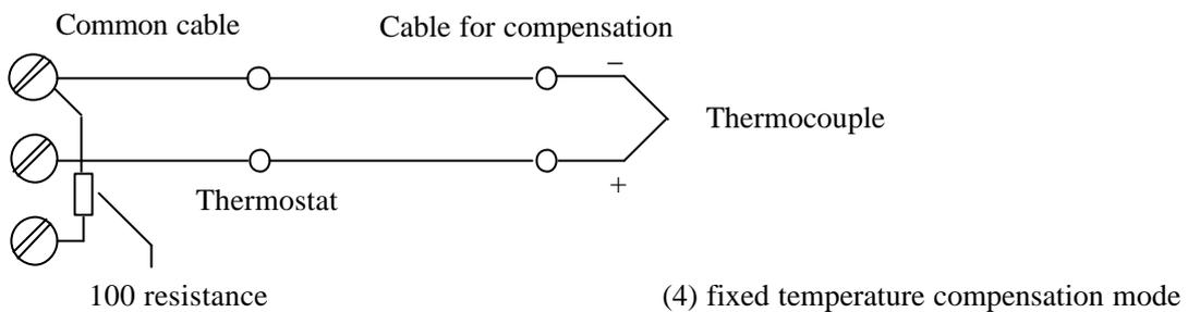
**Note : the temperture of thermostat should be controlled at 50**
