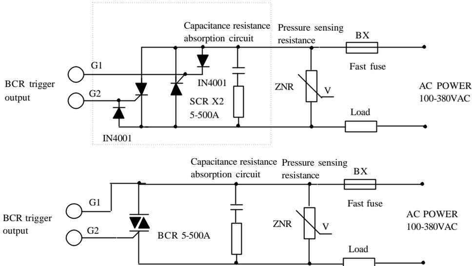
**Wiring diagram for BCR trigger output**
