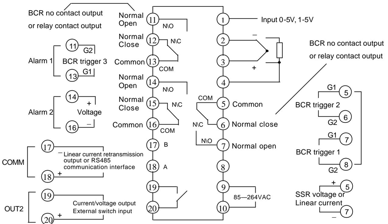
*96x96mm, 80x160mm, 48x96mm, Front panel specification and wiring diagram*
