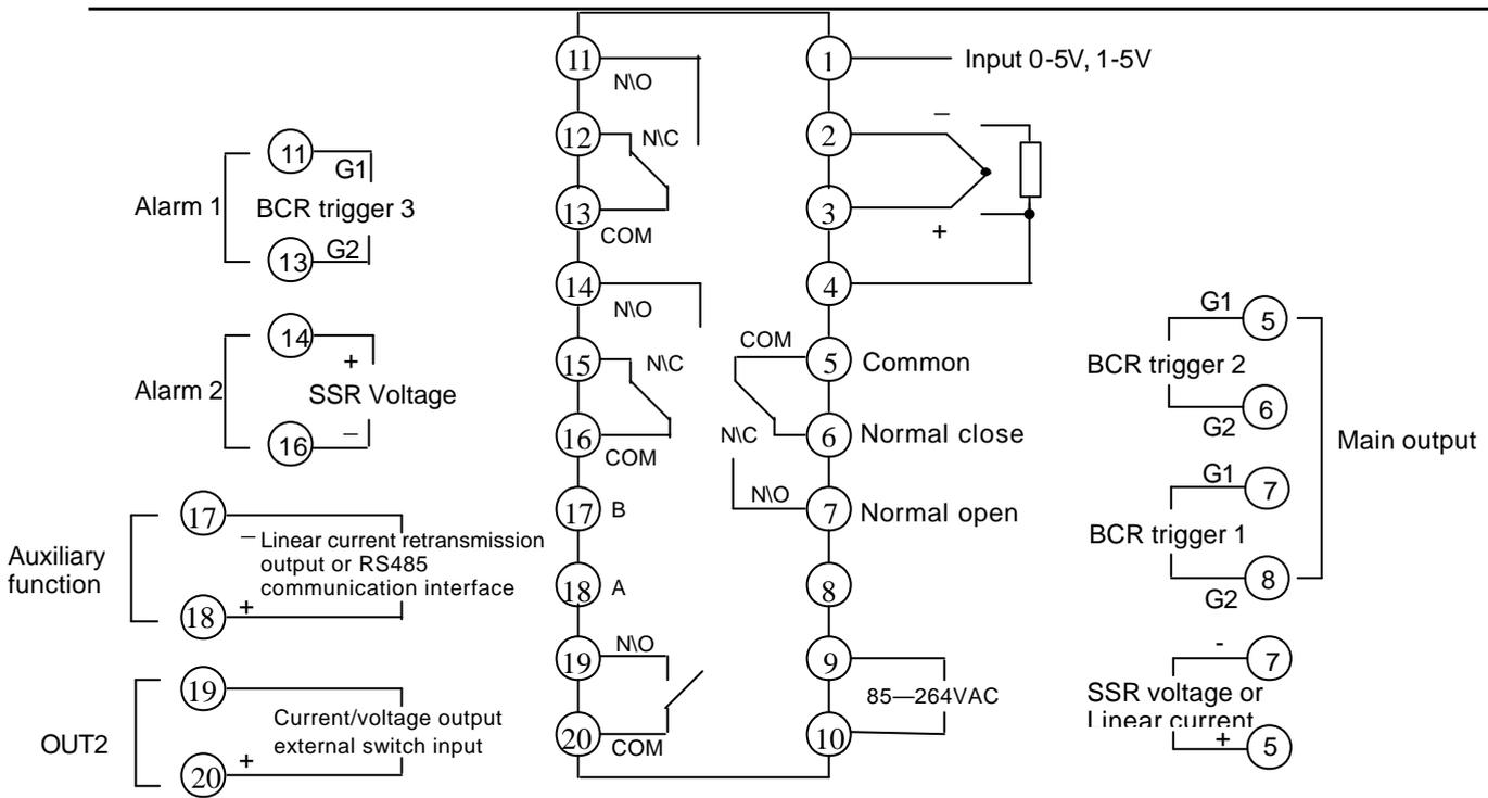
**160x80mm, 96x48mm, Front panel specification and wiring diagram**
